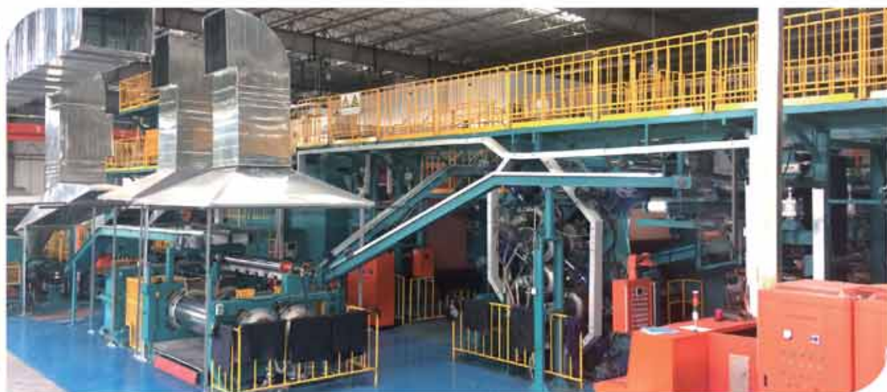
轮胎纤维帘布加张力压延生产线 TYRE FIBER CORD CALENDERING LINE WITH TENSION
